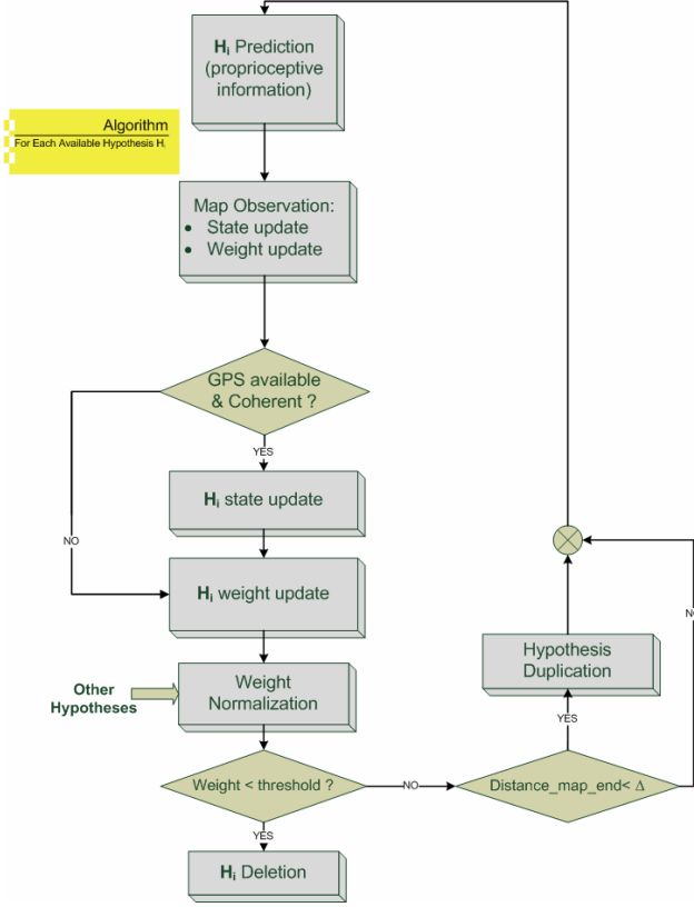
Fig. 3 Synoptic of MHMM
