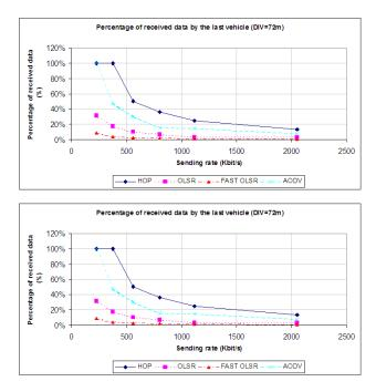
Fig. 7. Percentage of received data in the convoy with a crossing convoy and with an inter-vehicle distance equals to 27 m and 72 m.
