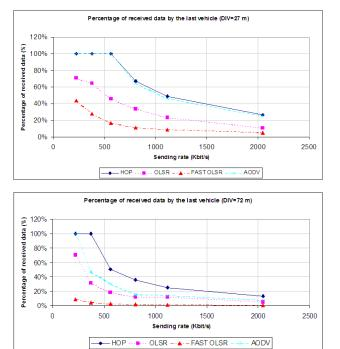
Fig. 9. Percentage of received data in the convoy with a perpendicular crossing convoy and with an inter-vehicle distance equals to 27 m and 72 m.
