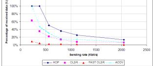
Fig. 5. Percentage of received data in the convoy with stopped vehicles (with an inter-vehicles distance equals to 27 m and 72 m).
