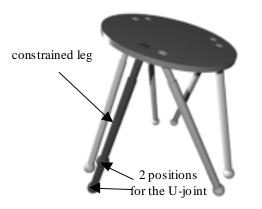
Figure 3: Two different robots with the same orientation of one leg for a given configuration q
