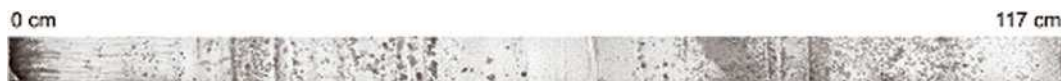
Fig. 3. Top 117 cm of the superimposed ice core, taken 1 km up-glacier from stake 6; 0 cm is at the previous summer surface. The different textures seen are due to varying air-bubble content (air bubbles are dark).
