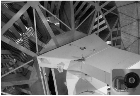
Figure 6. Cat Eye Reflectors at the telescope cabin.
