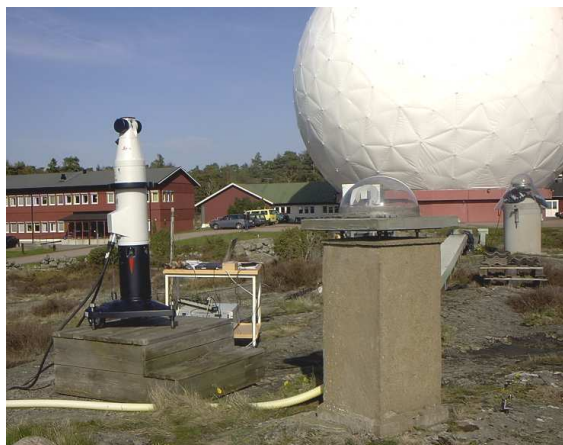
Figure 4. The laser tracker outdoors during the measurement of the traverse between the radio telescope enclosed by the white radome in the background and the GNSS monument in the foreground.
