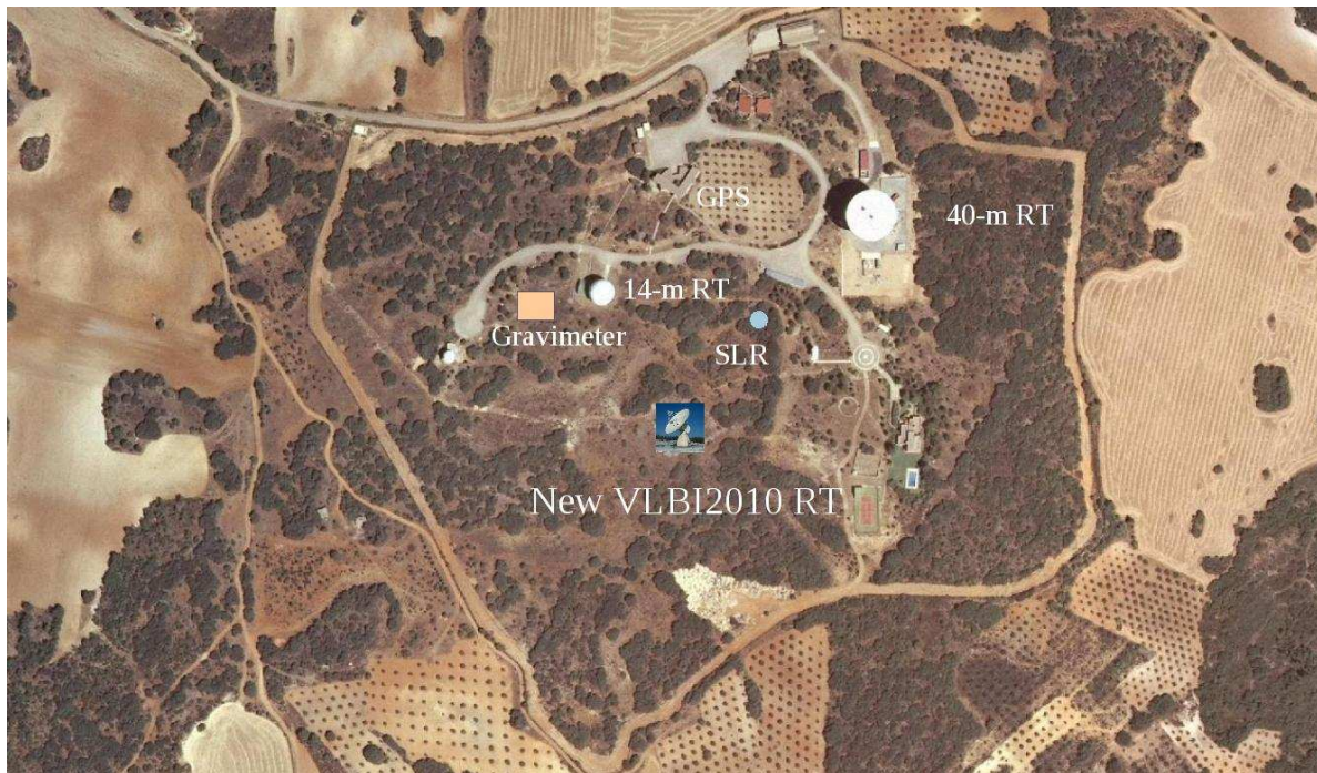
Figure 3. Possible placement of the geodetic instruments at the RAEGE station in Yebes (Spain).
