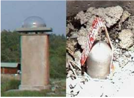
Figure 1. IGS-reference point (right) in the IGS-monument (left).
