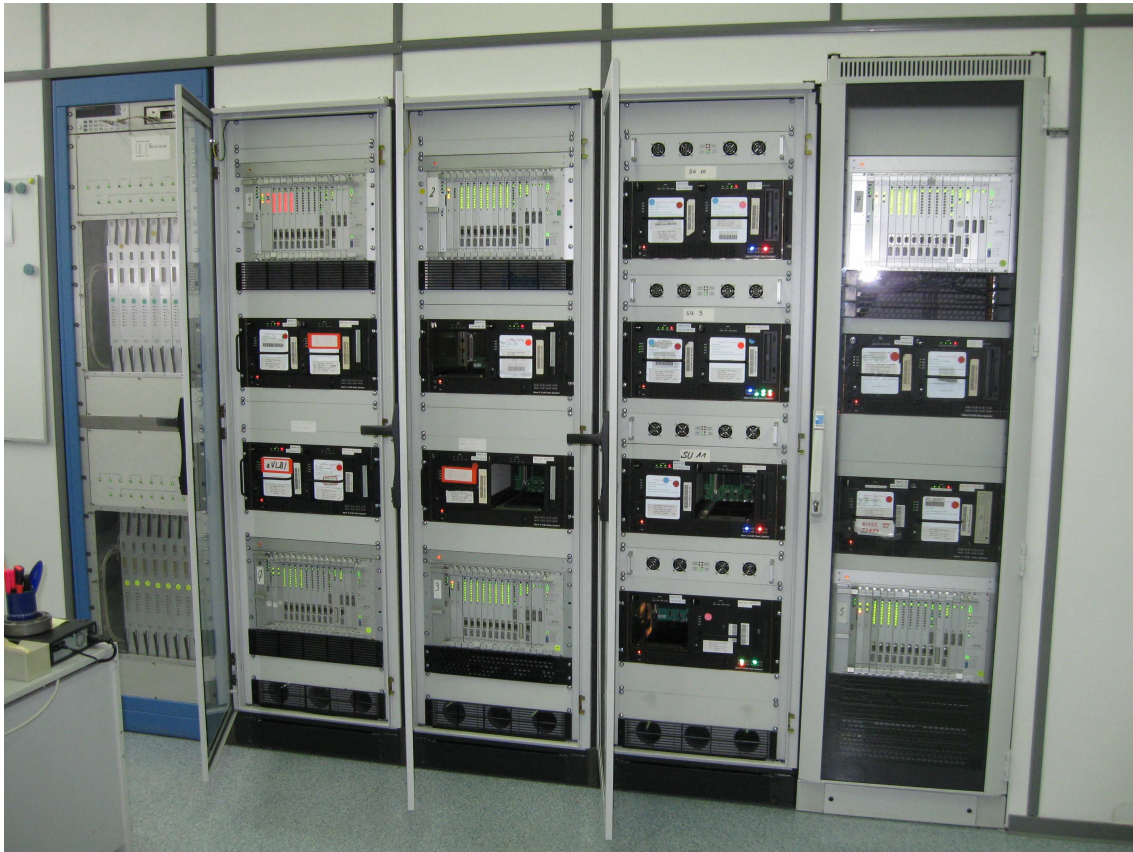
Figure 1. Picture of the MK IV correlator (left) with Mark 5As in 3 racks and 4 Mark Bs in one rack
