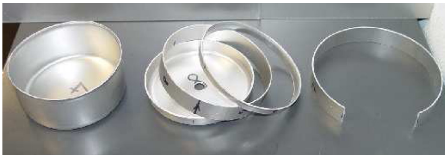
Fig. 17. From left to right, experimental drawn cup, cut rings and springback after splitting.
