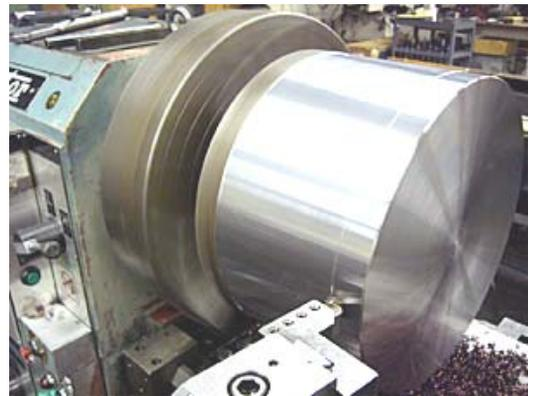
Figure 21: Turning operation
