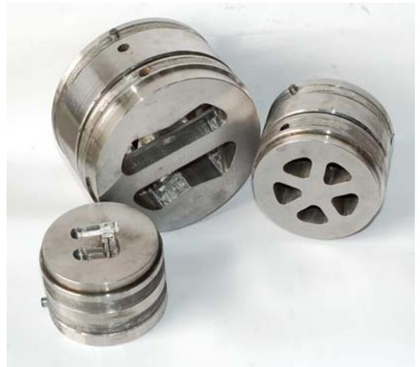
Figure 9: Aluminum extrusion dies
