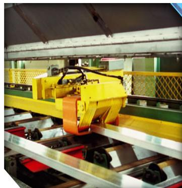
Figure 3: Run out table and puller
