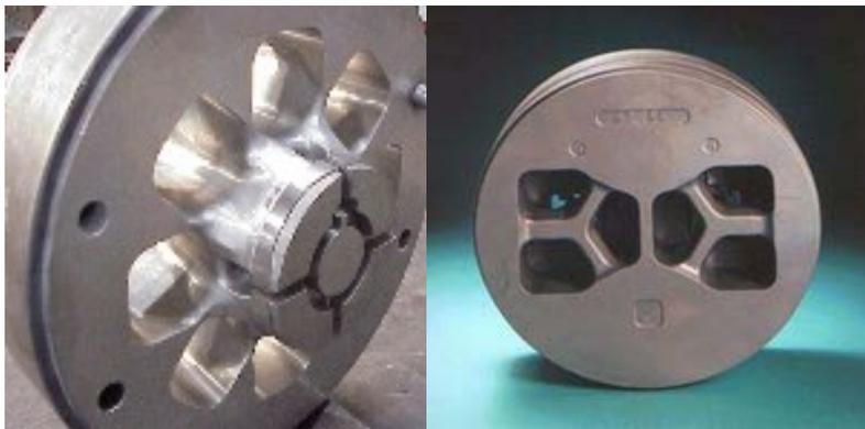
Figure 13: Typical hollow dies
