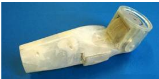
Fig. 4. Picture of the body part of the prosthesis with the elbow: use of Stereolithography process by Tech.Innovation society.
