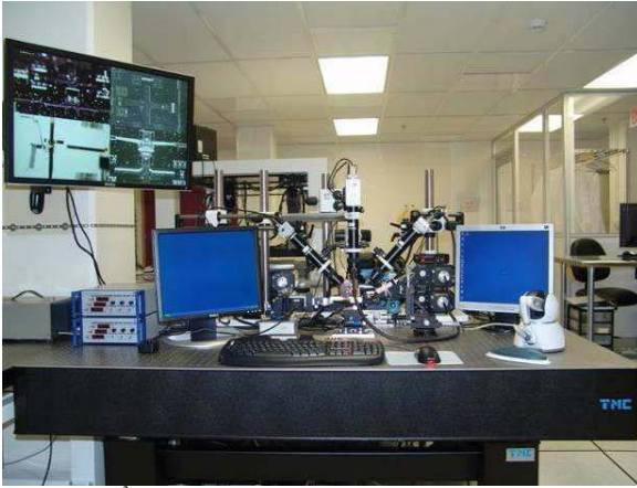
Figure 1: \mu^3 microassembly system at ARRI's Texas microfactory
