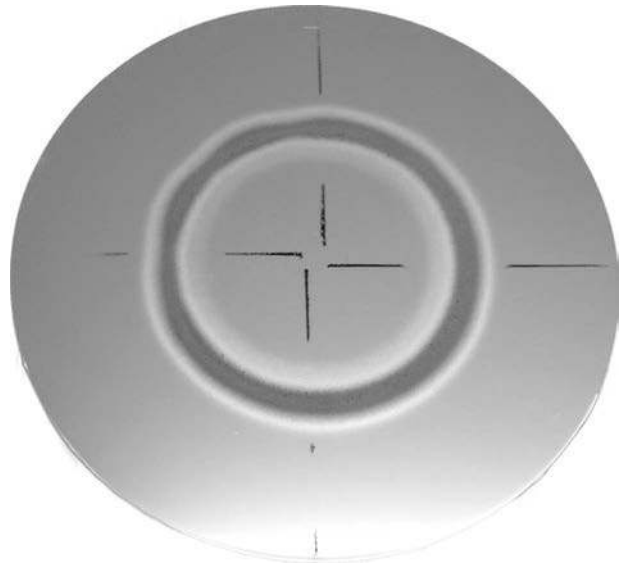
Fig. 16 Photograph of an eroded sample after an exposure time of 104 h. The external diameter of the sample is 100 mm. Operating conditions: V_c=65.3 m/s, p_u=21.3 bars, p_d=10.1 bars, and \sigma=0.9 .
