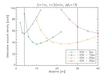
**Fig. 3.** Simulated performance of ALADDIN in terms of exozodiacal disc detection for four typical Darwin targets. The baseline design for ALADDIN has been used (see Table 3), assuming an integration time of 30 min, an uncertainty of 1% on the knowledge of the stellar angular diameter, and using the worst-case scenario for atmospheric turbulence (see text). The two vertical lines indicate the baseline range proposed for the ALADDIN conceptual design.
