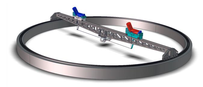
**Fig. 1.** Overview of the ALADDIN infrastructure. A 40-m rotating truss bearing the siderostats is mounted on a 30-m high structure (not represented). The light beams collected by the two siderostats are fed into off-axis telescopes and routed towards the nulling instrument cryostat by fixed relay optics (only five reflections outside the cryostat).
