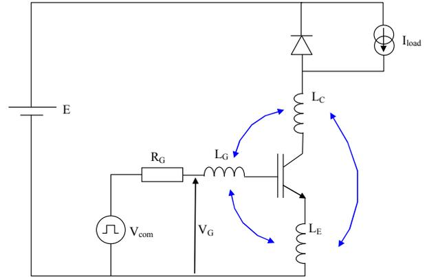
Figure 12: Representation of a switching cell for the power/drive interaction studies
