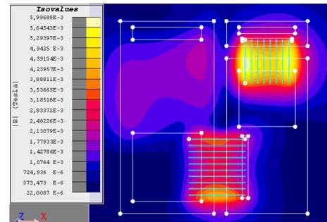
**Figure 16:** Induction of a classical buck converter
