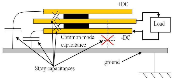
**Figure 21:** Equivalent electrostatic schematic of the 3D Chip on Chip module.
