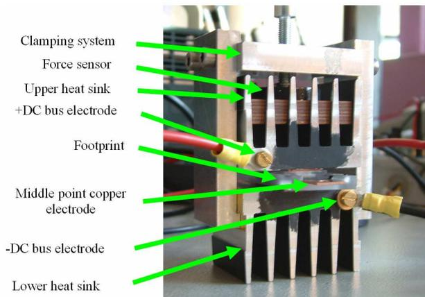
**Figure 6:** Single phase chip on chip power module
