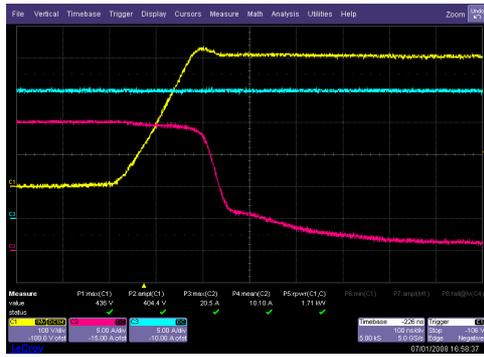
Figure 10: Switching waveforms of the buck converter
