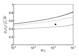
FIG. 6: Critical current divided by  $\sqrt{W/l_c}$  and normalized to  $I_0 = \lambda \sqrt{\sigma h/\rho_0 \alpha}$ , versus wire width for substrate thicknesses  $e/l_c = 0.5$  (thick line, optimal case), 10 (dashed line) and 0.01 (thin line). The point represents the case studied in this paper : a 200  $\mu$ m wide, 3  $\mu$ m high-wire on an AlN substrate of width  $e = 600 \ \mu$ m, for the parameters of Table 1. In this case,  $I_c = 16$  A.
