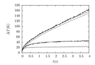
FIG. 3: Wire heating at long times for a 200  $\mu$ m wide-wire running a current of 5 A. Solid lines give the experimental results for, from top to bottom, a chip laid on paper, a chip maintained on a copper block with a pressure of  $2 \times 10^3$  Pa and a chip glued on the copper block. The other lines are theoretical predictions (see text).
