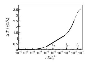
FIG. 2: Transient wire heating for  $W = 3 \times 10^{-3} l_c$  and  $e = 3 \times 10^{-2} l_c$  (dashed line). Temperature and time are scaled to  $\Phi/\lambda$  and  $t_c = l_c^2/D$  respectively. The solid lines correspond to fits with the functions (from earlier to later times)  $a_1 * \Delta T^{1Dz}$ ,  $\Delta T^{2D}$  and  $a_3 + b_3 \Delta T^{1Dx}$ , the fitted parameters being  $a_1 = 0.74$ ,  $W_{\text{eff}} = 0.17W$ ,  $a_3 = 1.0$  and  $b_3 = 0.79$ .
