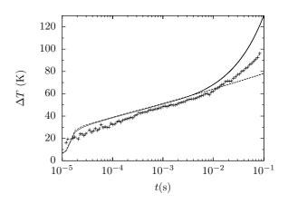
FIG. 4: Wire heating at long times for a 7  $\mu$ m wide-wire running a current of 1.7 A. Lines are predictions of the full model (solid) and the bare 2D model of Eq. 2 (dashed). The crosses are experimental data.
