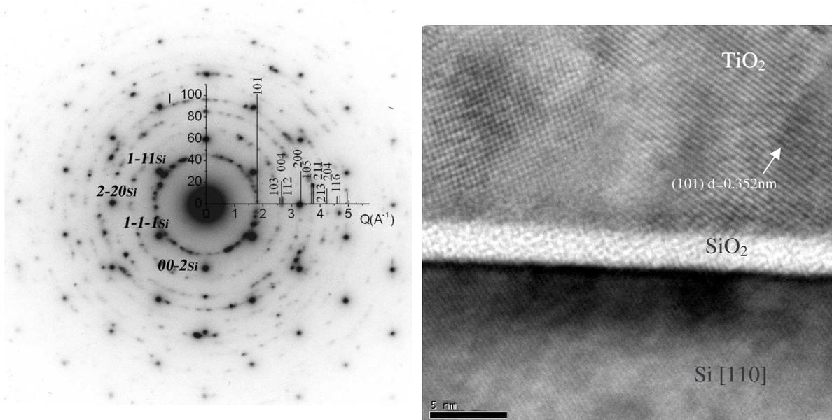
Figure 2 a) Indexation of the electron diffraction pattern of the layer  $\text{TiO}_2$  interface where the Si substrate is oriented along a  $[110]$  zone axis. B) High resolution image of the layer cross
