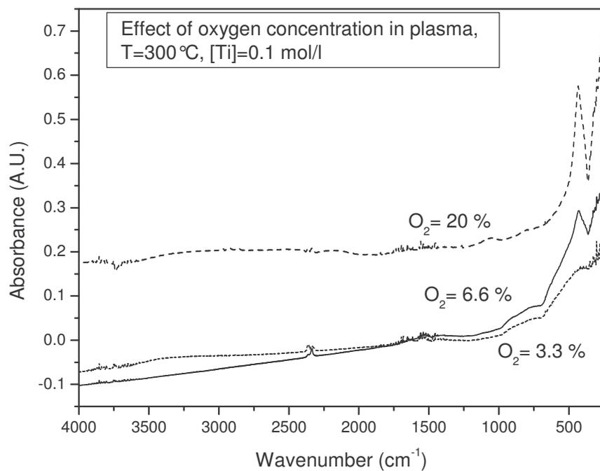
Figure 5 FTIR spectra of samples deposited from 0.1 mol/l TiO(acac)<sub>2</sub> solution with different oxygen concentration in plasma
