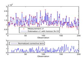
Fig. 4.  $x_1$  state estimation and measurement
