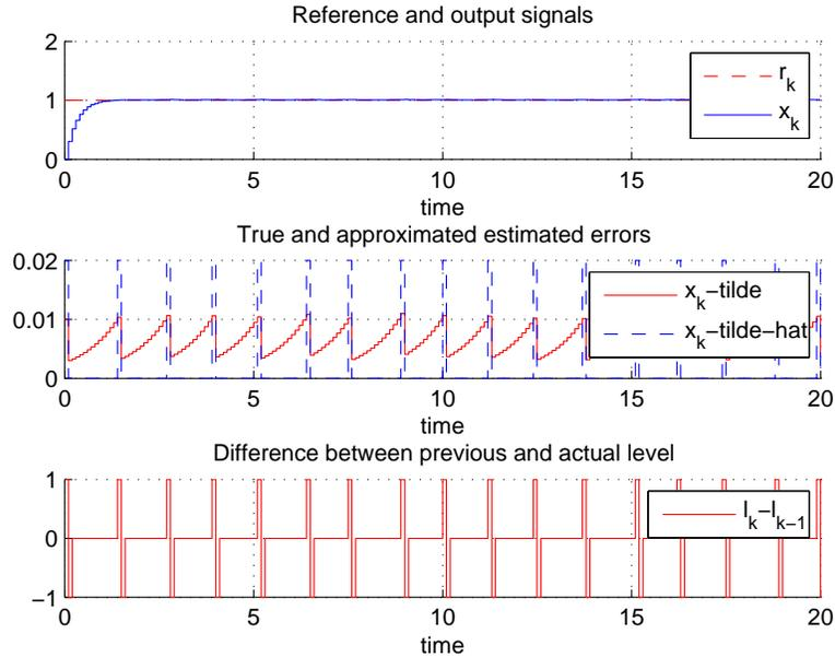
Fig. 4. Simulation results with  $\Delta = 0.02$  ;  $T_s = 0.05$  yielding  $|l_k - l_{k-1}| \leq 1$ . Output and reference (upper),  $\hat{x}$  vs.  $\tilde{x}$  (middle), and  $l_k - l_{k-1}$  (lower)
