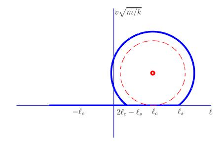
Figure 13. Phase plane for the hybrid model of stick-slip motion (see "Hybrid Model"). The sticking regime is the line  $2l_c - \ell_s \leq \ell \leq \ell_s$ . The slipping motion forms arcs of circles with center at  $(\ell_c, v_p \sqrt{m/k})$ , for v > 0. The center is marked with a circle. The dashed curve is a circle with center at  $(\ell_c, v_p \sqrt{m/k})$  and radius  $v_p \sqrt{m/k}$ . All trajectories starting outside this circle converge to the limit cycle.
