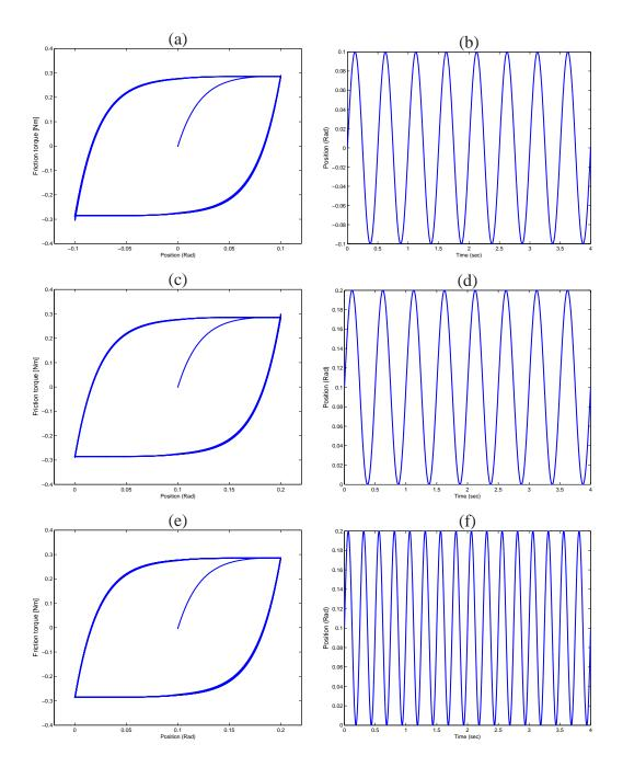
Figure 9. Illustration of the rate-independent property of the Dahl model. The left plots show phase planes while the right plots the position as a function of time. The input is sinusoidal with frequency 2 Hz in the curves (a) - (b). A bias at the inputs is added in the experiments shown in (c) and (d); the output is shifted but the produced path does not change. The plots (e) - (f)show that the limit cycle does remains the same when the frequency at the input is changed to 4 Hz.
