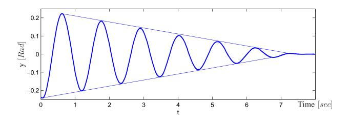
Figure 12. Oscillation of a pendulum supported by ball bearings. Notice that the amplitude decays linearly, indicating that ball-bearing friction is similar to solid friction.
