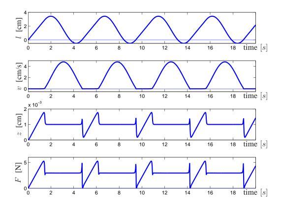
Figure 4. Behavior of the system in Figure 3 when the right hand side of the spring is pulled with constant velocity. The graph show the elongation of the spring l, the velocity of the mass v, the state z of the friction model, and the friction force F. The parameters are m = 1, k = 2,  $v_p = 2$ , and f = 0. The function g is given by (4) with parameters  $\alpha = 1$ ,  $\sigma_0 = 2900$ ,  $\sigma_1 = 107$ ,  $F_c = 2.94$ ,  $F_s = 5.88$  f(v) = 0, and  $v_s = 0.1$ .
