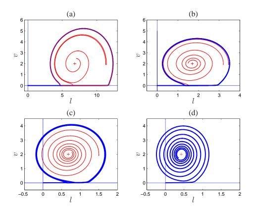
Figure 8. Change of behavior with spring coefficient k. The equilibrium shifts toward the left with increasing spring coefficient. For k = 2, (a) shows two red trajectories, one converges to the equilibrium the other converges to the limit cycle. As k increases, the region of attraction of the equilibrium increases as shown in (b) and (c). The limit cycle disappears when k is sufficiently large as shown in (d). The stiffness is (a) k = 0.5, (b) k = 2, (c) k = 5, (d) k = 8.
