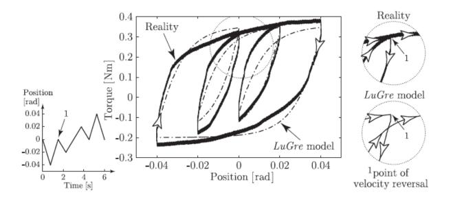
Figure 11. Experiments reported in [17] showing limitations at the LuGre model in predicting behavior at velocity reversals. The solid curve shows experimental data from a vertical electrodischarge machining axis. Figure reproduced with permission.
