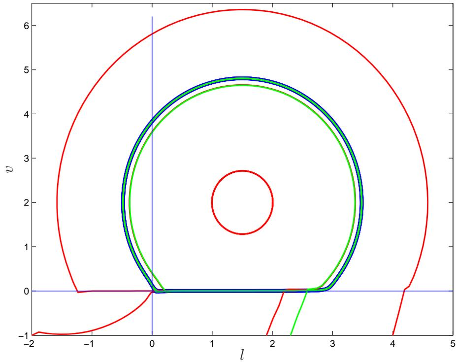
Figure 5. Projections of trajectories of the third-order system (14)-(16) on the  $v - \ell$  plane. The stick slip motion is the heavy blue line. All trajectories starting outside the blue line approach stick slip motion. Trajectories starting close to the equilibrium give sinusoidal nonsliding motion, whereas trajectories starting inside but close to the limit cycle converge to stick-slip motion.
