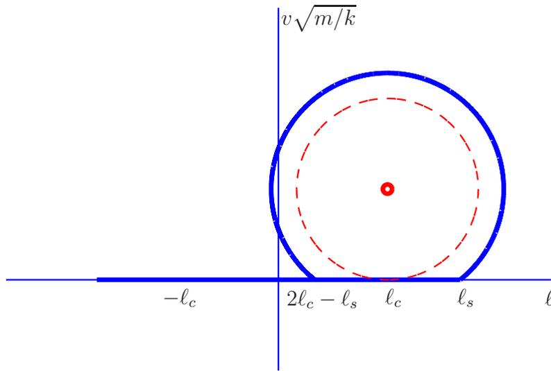
Figure 13. Phase plane for the hybrid model of stick-slip motion (see "Hybrid Model"). The sticking regime is the line  $2\ell_c - \ell_s \leq \ell \leq \ell_s$ . The slipping motion forms arcs of circles with center at  $(\ell_c, v_p\sqrt{m/k})$ , for  $v > 0$ . The center is marked with a circle. The dashed curve is a circle with center at  $(\ell_c, v_p\sqrt{m/k})$  and radius  $v_p\sqrt{m/k}$ . All trajectories starting outside this circle converge to the limit cycle.
