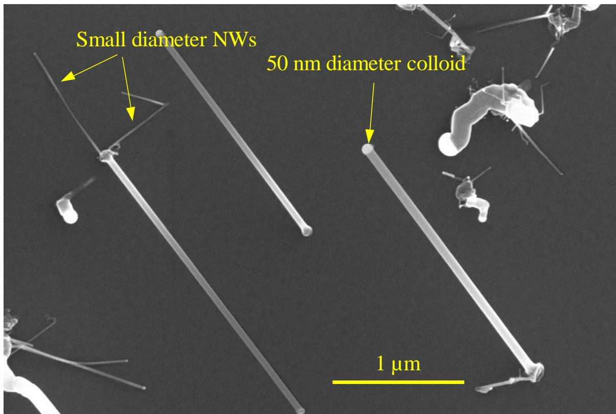
**Figure 7** SEM images of nanotrees grown from 200 nm diameter trunks. The branches are grown from gold droplets present on the trunk sidewall. In (a) we can see the overgrowth NW on the top with diameter reducing, in (b) zoom of nanotree.
