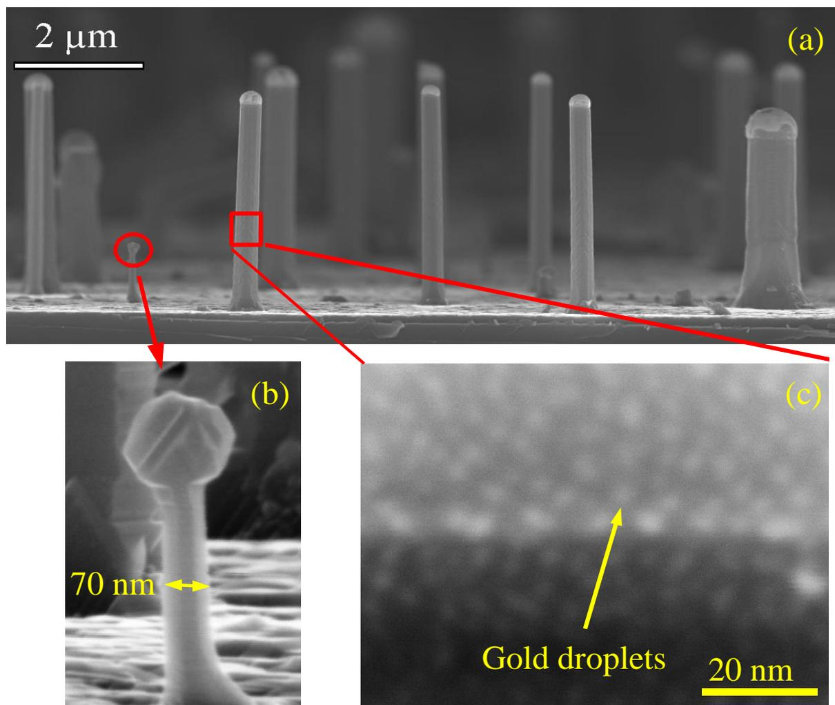
**Figure 2** SEM images of SiNWs grown from 50 nm gold colloids. a) growth at 600°C and silane 10 sccm. b) 550°C and silane 20 sccm. c) 450°C and silane 20 sccm.
