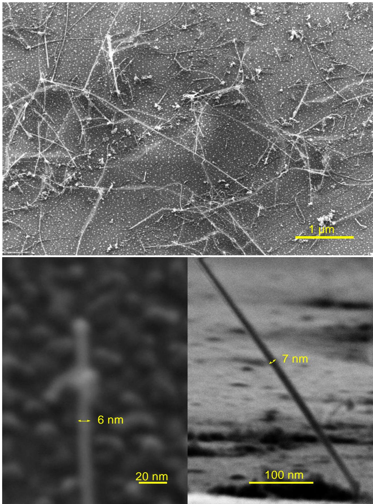
**Figure 6** SEM image of SiNWs grown from 50 nm diameter gold colloid catalyst at 430°C and 50 sccm silane. We can observe small diameter NWs (from 5 nm to 10 nm) at the base of the larger NWs.
