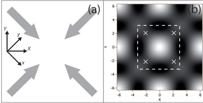
Figure 1. a) Layout of the laser beams. b) Spatial distribution of the intensity in the  $(X, Y)$  space. Black corresponds to the minimum value (zero intensity), while white corresponds to the maximum. The dotted square delimits the elementary mesh of the lattice, and the white crosses are the saddle points.
