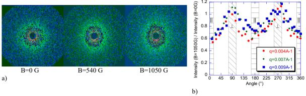
Figure 5: Deformation of hollow magnetic shells (system B 1eq) studied by anisotropic SANS.
