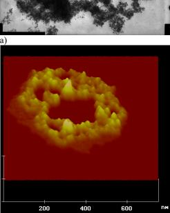
membrane made of PB<sub>48</sub>-b-PGA<sub>56</sub> and 1 equiv. of S2-CH<sub>2</sub>Cl<sub>2</sub>. The scale bar measures 333 nm. b) 3-d view built from an AFM picture of the same sample (see Supplemental Information II) showing a flat copolymer membrane stuffed with magnetic iron oxide nanoparticles. Strong spreading on mica opens holes in the central part, whereas some pure copolymer bilayer is visible at the periphery.
