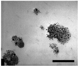
Figure 2: TEM picture of hybrid copolymer micelles loaded with magnetic nanoparticles
