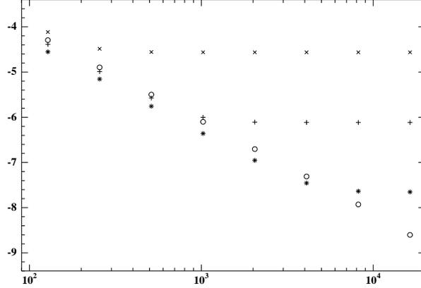
Figure 4: Numerical errors  $\|u_{N,N_g} - u\|_{H^1}$  ( $\times$ ),  $\|u_{N,N_g} - u\|_{L^2}$  ( $+$ ),  $\|u_{N,N_g} - u\|_{H^{-1}}$  ( $*$ ), and  $|\lambda_{N,N_g} - \lambda|$  ( $\circ$ ), for  $N = 30$ , as functions of  $N_g$  (in log scales).
