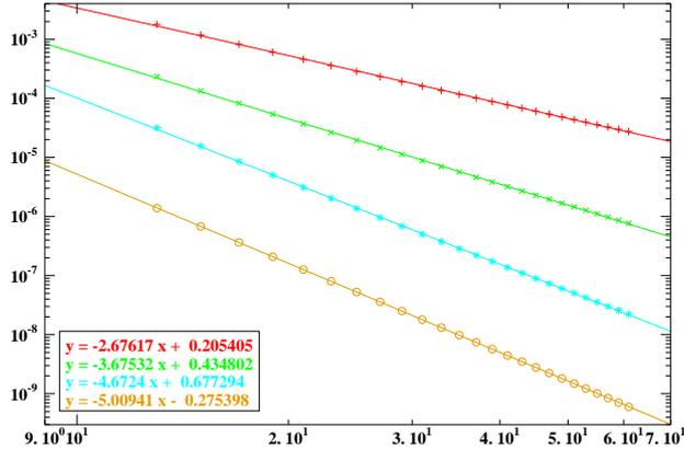
Figure 1: Numerical errors  $\|u_N - u\|_{H^1}$  (+),  $\|u_N - u\|_{L^2}$  (×),  $\|u_N - u\|_{H^{-1}}$  (\*), and  $|\lambda_N - \lambda|$  (o), as functions of  $2N + 1$  (the dimension of  $\tilde{X}_N$ ) in log scales.
