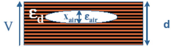
Figure 17: Simplified representation of a cavity in a sample
