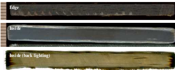
Figure 15 : Scan of an aged Class-H sample (740 h, 180°C, 2.3 bar O 2 )
