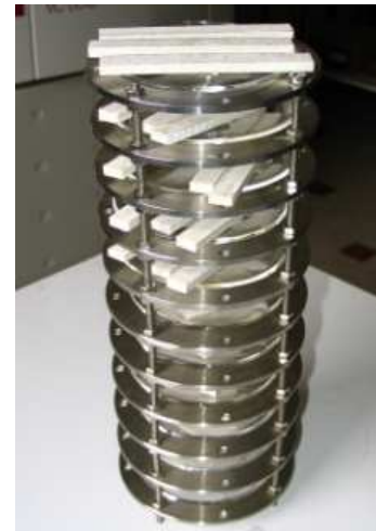
Figure 3: Stainless steel rack with glass plates and samples
