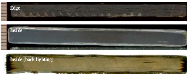
Figure 15 : Scan of an aged Class-H sample (740 h, 180°C, 2.3 bar O 2 )
