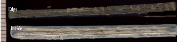
Figure 13: Scan of an aged HC-F sample (4250 h, 155°C, 2.3 bar O 2 )
