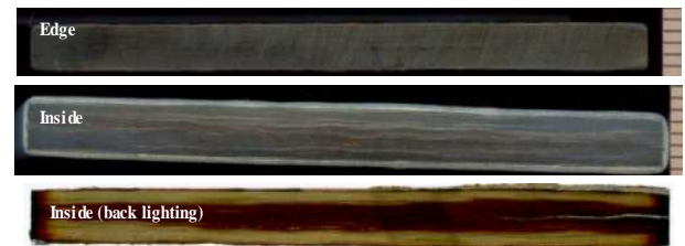
Figure 11: Scan of an aged Ref-F sample (805 h, 155°C, 2.3 bar O 2 )
