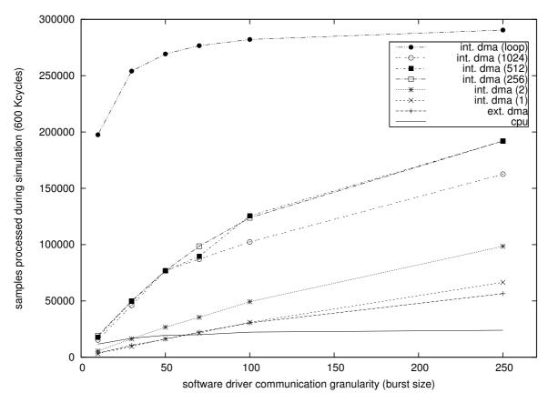
Figure 8. Hardware accelerator throughput according to different burst length and CPU or DMA communication mechanism
