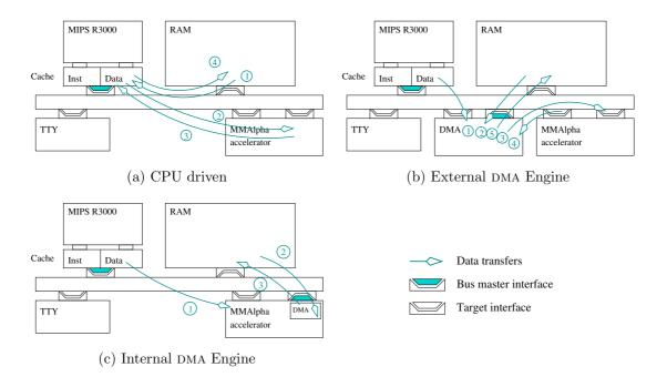
Figure 1. The three main interface modes: (a) CPU driven, (b) external  ${
