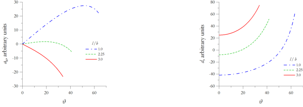
Figure 11. Left: lever arm of the buoyancy force for a floating rectangle of width l and immersion depth b vs. the angle of heel. Right: metacentric height. The \vartheta -values are limited by the requirement that of two angles of the rectangle be immersed. For l/b = 1 one always has an overturning moment, for l/b = 2.25 the moment is an overturning one for heel angles less than \vartheta \approx 31^\circ and becomes a restoring one at larger \vartheta . For l/b = 3 one always gets a restoring moment.
