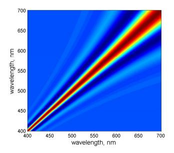
**Fig. 7.** Cross-correlation function (Eq. 10) of the spectrometer pixels at  $30 \, \text{km}$ , obliquity  $\sim 30^{\circ}$
