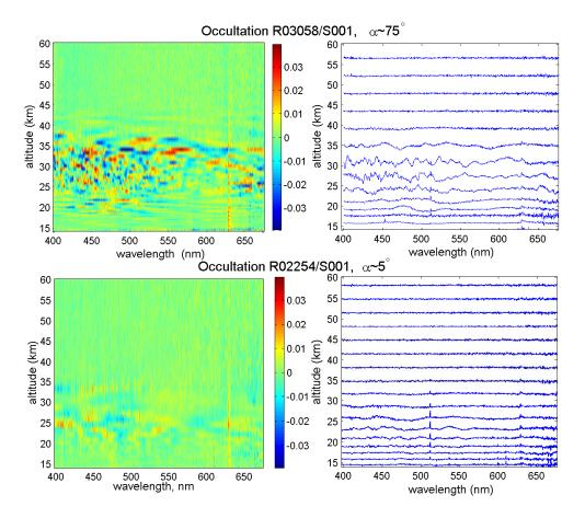
Fig. 5. Top: residuals in the oblique occultation of Sirius R03058/S001 ( $\alpha$ ~75°). Bottom: residuals in close to vertical occultation of Sirius R02254/S001. Left: color plot; right: scaled residuals (by the factor 50) at selected altitudes.
