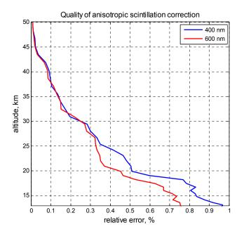
**Fig. 3.** Relative error in estimated transmittances caused by error of anisotropic scintillation 3 correction: results of Monte Carlo simulations.
