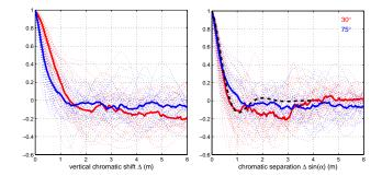
**Fig. 6.** ACF of residual fluctuations as a function of vertical chromatic shift (left) and as a function of chromatic distance x (right), for two series of sequential occultations of Sirius: with obliquities  $\sim$ 75° and  $\sim$ 30°. The altitude is 30 km. Bold lines: median. The dashed bold line in the right subplot indicates the parameterization given by Eq. (10).
