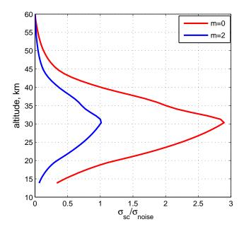
**Fig. 9.** Altitude dependence of ratio  $r = \frac{\sigma_{sc}}{\sigma_{\text{noise}}}$  at  $\lambda = 500$ nm, for stars of magnitude 0 and 2 and effective temperature  $T = 11\,000$  K. The obliquity of the occultation is  $\alpha = 30^{\circ}$ .
