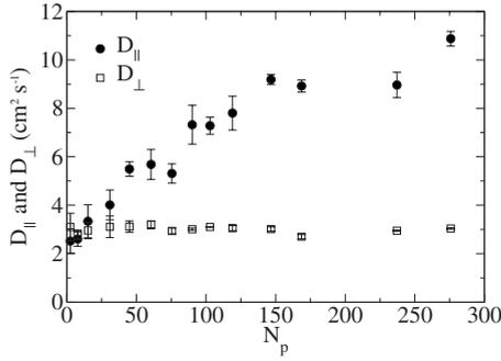
FIG. 11. Evolution of dispersion coefficients versus  $N_p$  for a size ratio  $D/d=10$ . These results have been obtained with  $H/D=14$ ,  $D=20$  mm,  $e_1=0.84$ , and  $e_2=0.99$ . Error bars are also represented.
