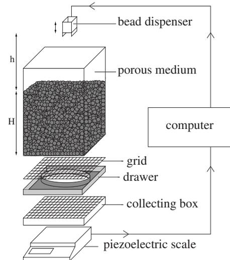
FIG. 1. Schematic description of the experimental setup. The small bead dispenser is placed at  $h$  from the top of the porous media of an height  $H$ . The collecting box is put on the scale.
