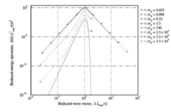
FIG. 3. Reduced energy spectra  $E(k,t)t^2/L_{expt}^3(t)$  (n=4) at the same times as a function of reduced wave number  $kL_{expt}(t)$ .
