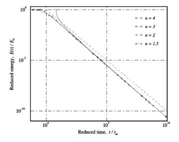
FIG. 7. Evolution of the computed integral energy E(t) for n = 1.5, 2, 3, 4 (dotted lines) compared to the theoretical leading-order prediction  $E(t)=L^2(t)/t^2$  (12) (solid line) and the same without the logarithmic correction (dashed line).
