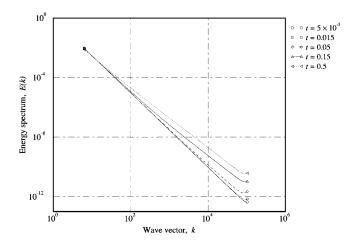
FIG. 18. Evolution of the energy spectrum with an initial spectrum proportional to  $|k|^{-2.5}$ . One can see that the amplitude of the high-frequency components *increases* with time, the  $|k|^{-2.5}$  spectrum transforming to a  $k^{-2}$  tail, whose energy really comes from the smallest wave-number components. These have a very slightly decreasing amplitude, so that the global energy is nearly constant, but slightly decays in time.
