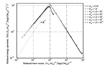
FIG. 5. Reduced energy spectra  $E(k,t)t^2/L^3(t)$  at the same times as a function of reduced wave number kL(t) using the theoretical value  $L(t) = (t/t_{\rm n})^{1/2} [\ln(t/2\pi t_{\rm n})]^{-1/4}$ .
