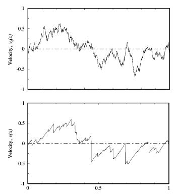
FIG. 16. Evolution of the velocity field for one particular realization with an initial spectrum  $k^{-2}$ . The upper plot is the Gaussian Brownian motion initial condition at t=0 and the lower plot is the velocity field at t=0.15, just before the decay of the smallest wavenumber component. Both signals have the same power spectrum. Note that the largest scales are nonlinearly distorted, but their amplitude is globally preserved, illustrating the principle of the persistence of large eddies.
