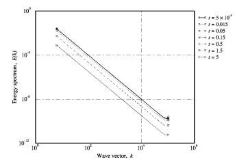
FIG. 15. Evolution of the energy spectrum with an initial spectrum proportional to  $k^{-2}$ . One can see that the spectrum does not change at all until the nonlinear time of the smallest wave-number component is reached (near  $t \approx 0.15$ ).
