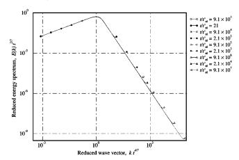
FIG. 9. Reduced energy spectra  $E(k,t)t^{2/7}$  (n=0.5) at the same times as a function of reduced wave number  $kt^{4/7}$ . Same conditions as in Fig. 8.
