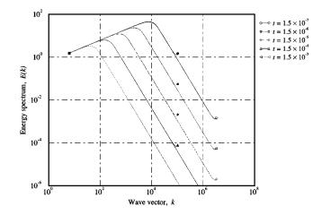
FIG. 8. Evolution of the energy spectrum with an initial spectrum proportional to  $|k|^n$  (n=0.5) at small wave numbers k. Resolutions  $N=2^{15}$  and  $N'=2^{20}$  are denoted by solid or open symbols, respectively. The labels correspond to output times  $t_1=1.5 \times 10^{-7}$ ,..., up to  $t=1.5 \times 10^{-3}$  (in absolute time, the reduced time  $t/t'_{nl}$  depends on the value of the upper cutoff  $k_u$ , equal in this case to  $N\pi$  or  $N'\pi$ ).
