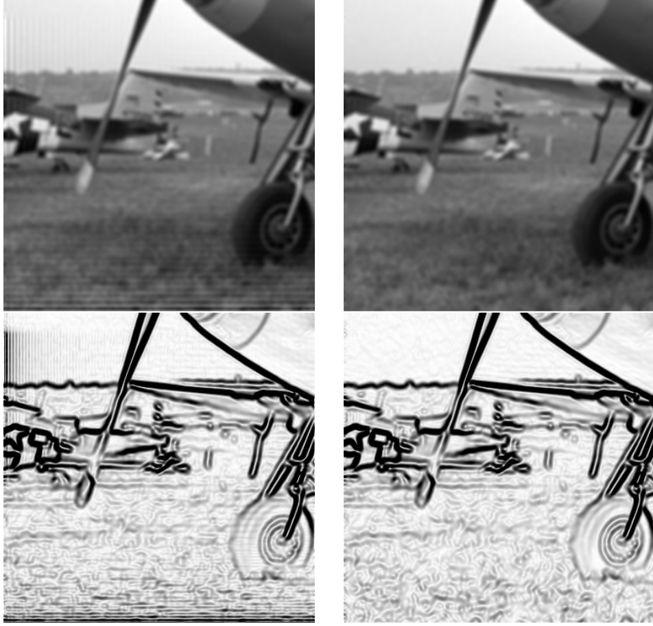
Figure 5: First row: the bottom-left corner of the Plane image (see Figure 4) has been zoomed by a factor 4 by applying a periodic cardinal sine (sinc) interpolation. The sinc interpolation was applied in two different ways: on the left column, directly to the Plane image; on the right column, to the periodic component only, the smooth component being processed with bilinear interpolation. As we can see, the ringing artifacts caused by periodic sinc interpolation (or equivalently, by the use of the DFT), are completely avoided when the periodic plus smooth decomposition is used. The effect is particularly strong on the image gradient (norm), displayed under each image (second row). This illustrates the fact that periodic plus smooth decomposition offers a way to use Shannon (sinc) interpolation without undergoing unpleasant edge effects.
