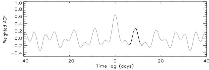
**Fig. 6.** Weighted autocorrelation function of the out-of-transit light curve (gray line). We estimate the rotation period of the star using a Gaussian fit to the peak of the first side-lobe (dashed black line).
