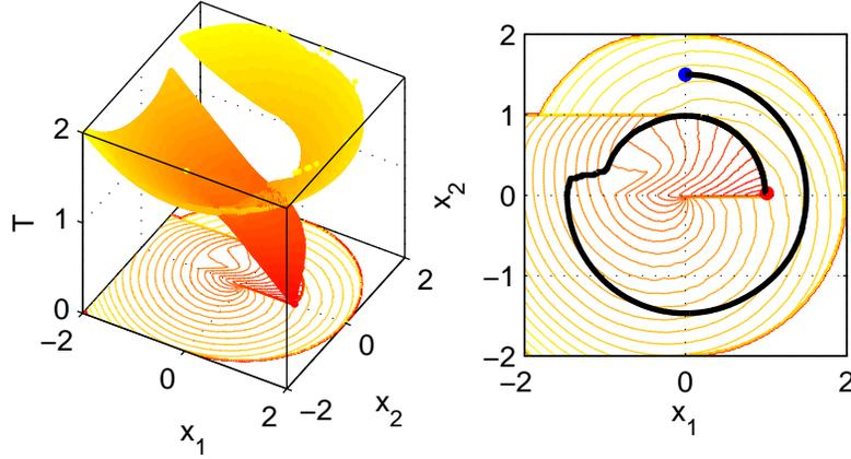
Figure 1: Example 1, 3d view of  $(x_1, x_2, T(x_1, x_2))$  (left) and isovalues of  $T$  with an optimal trajectory reconstruction (right).
