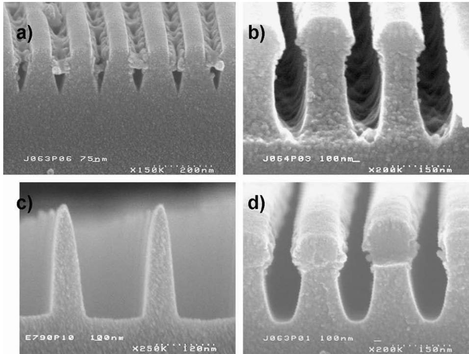
**Fig. 11.** Porous SiOCH trenches etched with different plasma parameters (a) lower pressure (50 mTorr), (b) 7 sccm  $\text{CH}_2\text{F}_2$  addition, (c) higher source power (600 W), (d) dense SiOCH trenches.
