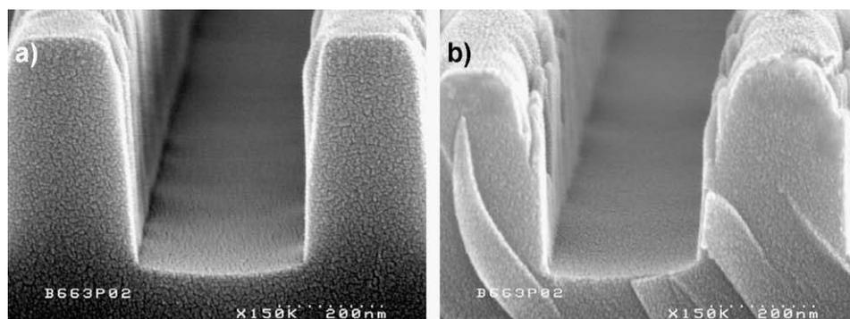
Fig. 7. SEM picture of SiO<sub>2</sub> trenches patched on a TiN / SiO<sub>2</sub> wafer (a) before etching, (b) after etching.
