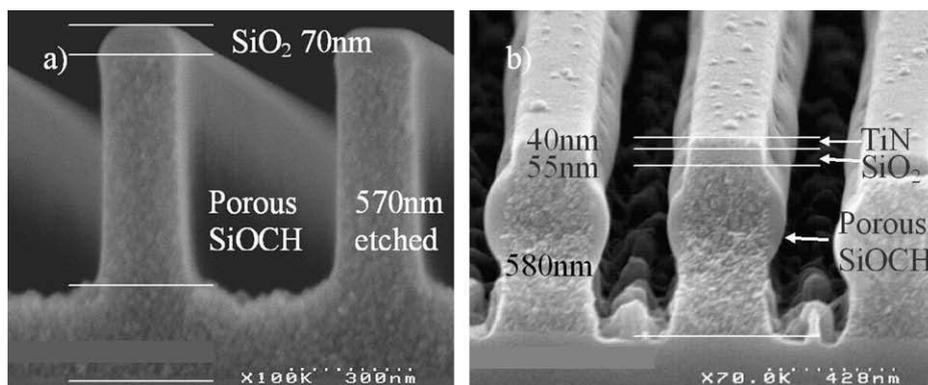
Fig. 5. Porous SiOCH trenches etched with (a) a SiO<sub>2</sub> hard mask, (b) a TiN hard mask.
