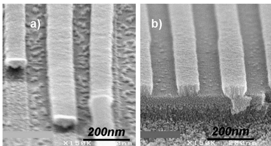
**Fig. 3.** SEM pictures after hard mask opening (BT + ME + stripping) with different BT: (a) pure Ar plasma, (b) with Cl<sub>2</sub> addition in the Ar plasma.
