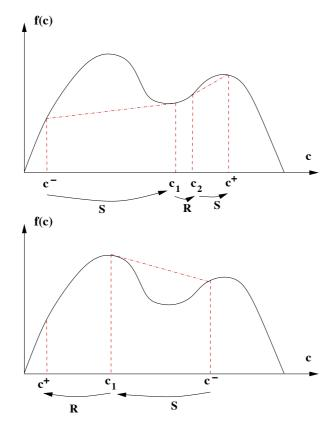
Fig. 4.2. shocks chords are shown as dashed lines. On the left  $c^-$  is connected to  $c^+$  via a shock (S), a rarefaction wave (R) and a shock. On the right,  $c^-$  is connected to  $c^+$  via a shock and a rarefaction wave.
