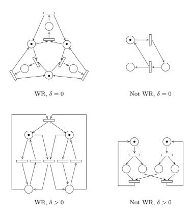
Fig. 3. Deficiency zero and weak reversibility are independent.
