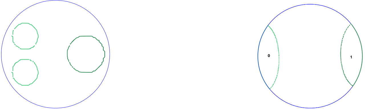
F 1. Initial and optimized level sets for a problem with two constraints
