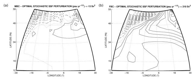
FIG. 13. Optimal stochastic perturbations for the (a) MBC and (b) FBC experiments. The maximum of the SSF structure is normalized to 1 psu yr<sup>-1/2</sup>. Perturbations induce a variability of the circulation intensity with a std dev of 3.6 and 14.5 Sv, respectively; CI is 0.05 psu yr<sup>-1/2</sup>.
