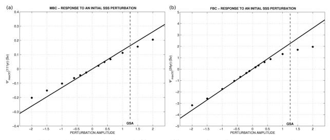
FIG. 12. Validation of the linear approximation for the (a) MBC and (b) FBC experiments: linear theoretical values of the response of the MOC intensity (solid line) are compared to the nonlinear model time integrations (+) for perturbation amplitudes from -2 to +2 psu. The relative error for GSA is less than 15% (30%) for the MBC (FBC) experiment. Note the much larger response in the latter case.
