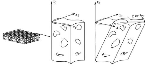
Fig. 2. Kelsey et al. unit load method
