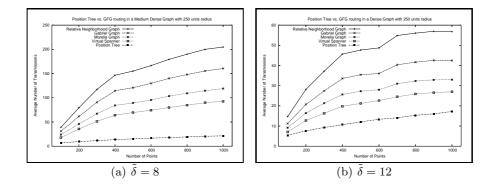
Fig. 5: Average path length (in # of hops) for  $\tilde{\delta} = 8$  and  $\tilde{\delta} = 12$  for RTP and GFG using several planarization methods, for R = 0.25.
