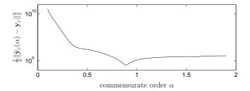
Fig. 5. Criterion to minimize with respect to  $\alpha$  for a data set with SNR=20 dB (true commensurate order: 0.9)
