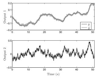
Fig. 1. Output data  $\mathbf{y}$  and output of the estimated model  $\hat{\mathbf{y}}$  for a PRBS as input (SNR=20 dB).
