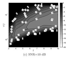
Fig. 3. Normalized error norm  $\|\hat{y} - y\|_2/\|y\|_2$  in dB versus the number of block rows i and the filter frequency  $\omega_f$  for various SNRs.
