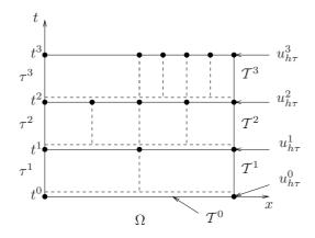
FIG. 2.1. Time-dependent meshes and discrete solutions
