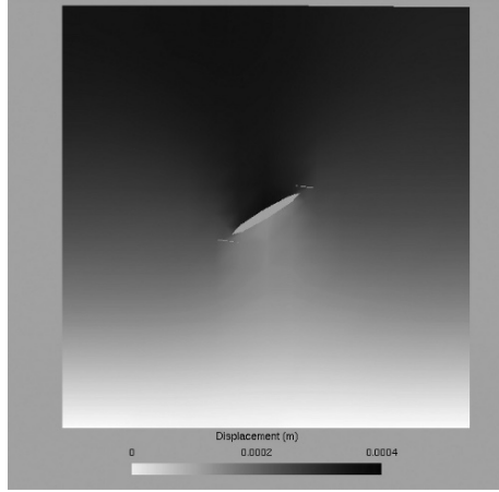
Figure 5. Deformed mesh for a crack angle of 30^\circ (magnified \times 1000 )
