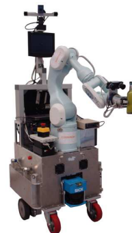
Figure 7: Our robot Jido composed of a mobile base and a 6 dof arm
