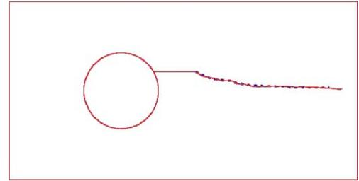
Fig. 13. Comparison of calculated (continuous lines) vs. experimental (dotted lines) crack's paths.
