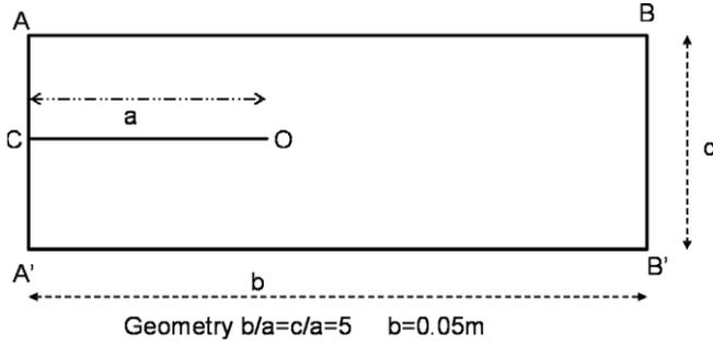
Fig. 3. DCB geometry.
