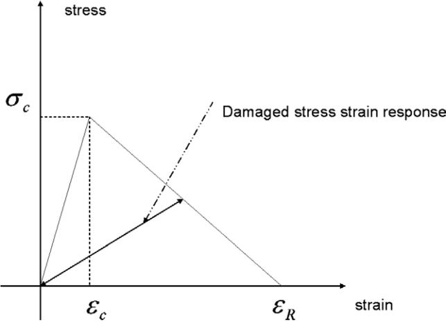
Fig. 1. Typical stress–strain curve for a brittle material.
