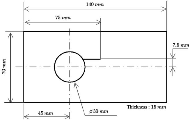
Fig. 8. Geometry of the PMMA specimen tested.
