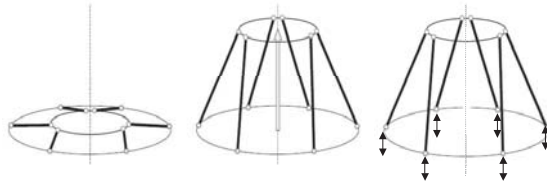
Fig. 1 Stowage, deployment, and correction stages.
