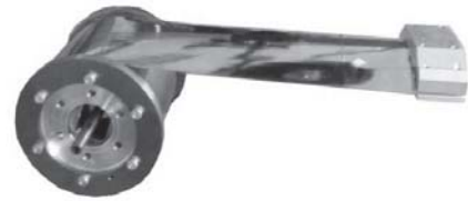
Fig. 2 A tape-spring coiling device.
