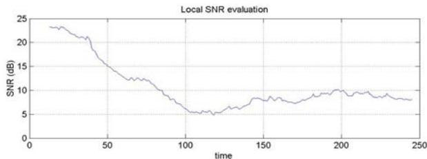
Fig. 9: Local SNR (dB) computed on 25 samples gliding window for a global SNR=15 dB
