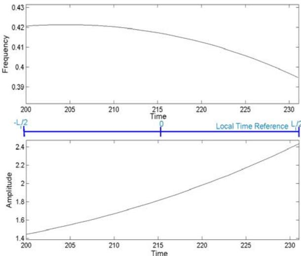
Fig. 2. Local segment of an AM/FM modulation (31 samples).
