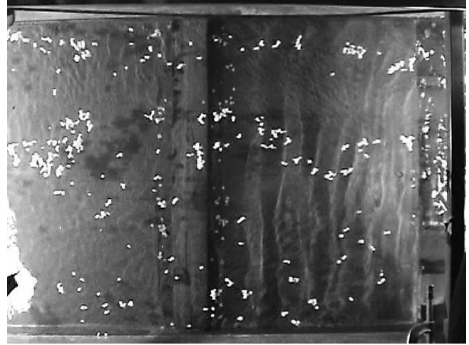
Fig. 2 Image extracted from a video sequence used for the experiment. Paper confetti transported on the water surface (from left to right).
