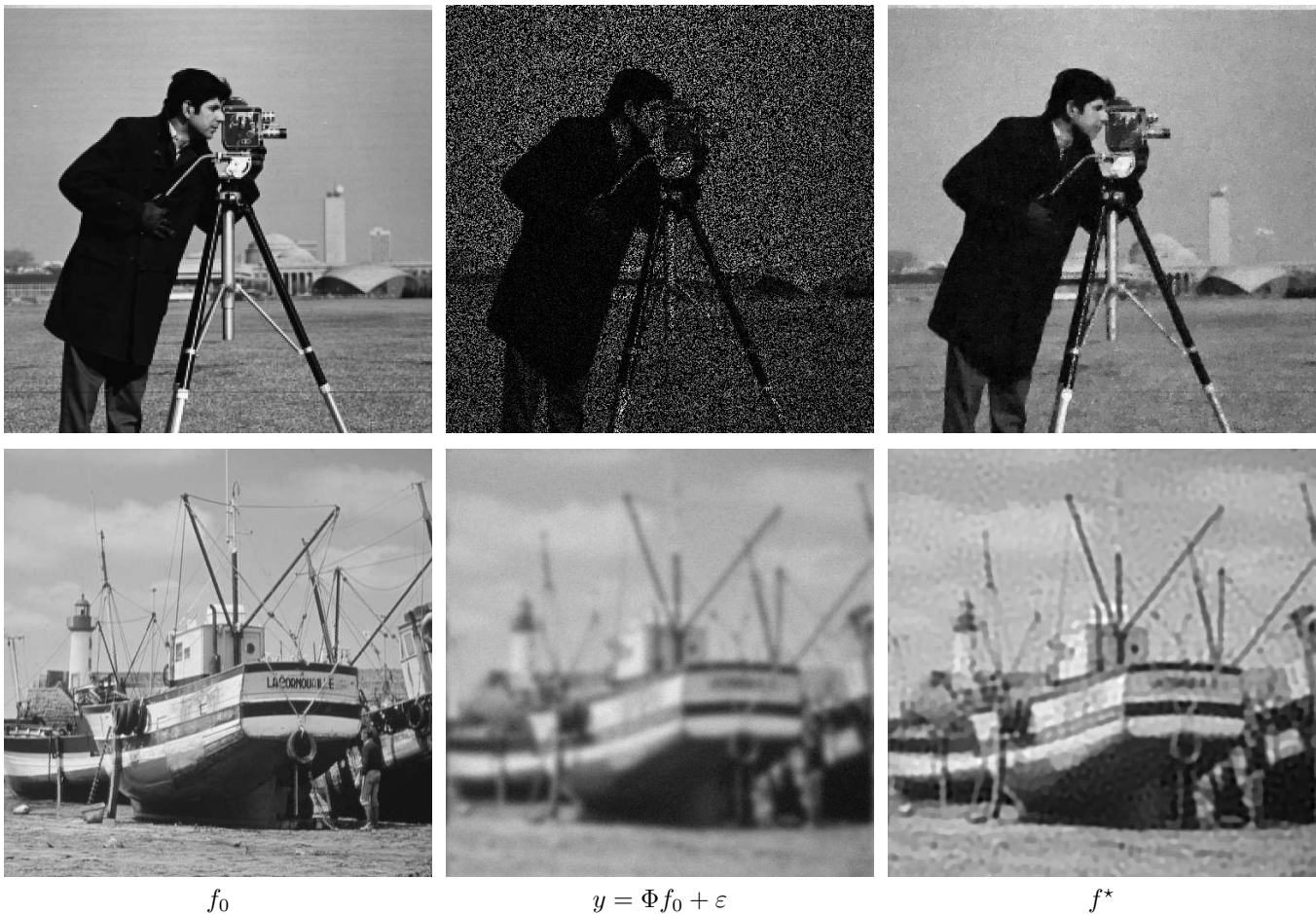
Fig. 5. Examples of inpainting (first row) and deconvolution (bottom row) using the TV constraint.
