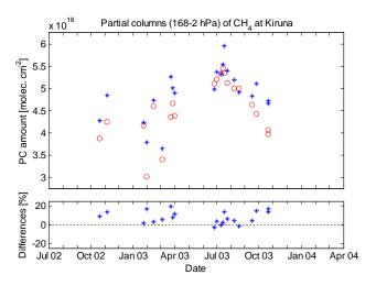
**Fig. 14b.** Time series of CH<sub>4</sub> partial column comparisons. Upper panel: ground-based FTIR (circles) and MIPAS v4.61 (stars) CH<sub>4</sub> partial columns for collocated measurements at Kiruna. Lower panel: relative differences between ground-based FTIR and MIPAS partial columns.
