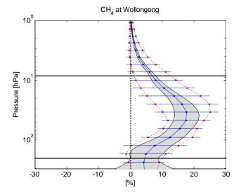
**Fig. 15d.** Statistical means and standard deviations of the relative differences mean(MIPAS-FTIR)/mean(FTIR) [%] of the CH<sub>4</sub> profiles measured at Wollongong. The shaded areas correspond to the estimated random error on the relative differences. The two black horizontal bars show the pressure ranges used for the partial column comparisons of Table 3. The statistics shown is for the  $\pm 4$  h and  $\pm 400$  km coincidence criteria.
