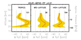
**Fig. 13.** Comparison of MIPAS  $N_2O$  v4.61 profile with ASUR. The differences ( $\Delta$  VMR=ASUR VMR - MIPAS VMR) are averaged over the tropics ( $5^{\circ}$  S- $30^{\circ}$  N), mid-latitudes ( $30^{\circ}$  N- $60^{\circ}$  N), and high latitudes ( $60^{\circ}$  N- $90^{\circ}$  N). Shaded area is the standard deviation of the profiles averaged.
