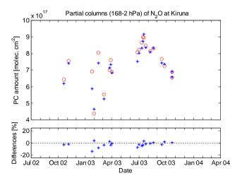
**Fig. 16b.** Time series of  $N_2O$  partial columns comparisons. Upper panel: ground-based FTIR (circles) and MIPAS v4.61 (stars)  $N_2O$  partial columns for collocated measurements at Kiruna. Lower panel: relative differences between ground-based FTIR and MIPAS partial columns.
