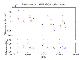
**Fig. 16e.** Time series of  $N_2O$  partial columns comparisons. Upper panel: ground-based FTIR (circles) and MIPAS v4.61 (stars)  $N_2O$  partial columns for collocated measurements at Lauder. Lower panel: relative differences between ground-based FTIR and MIPAS partial columns.
