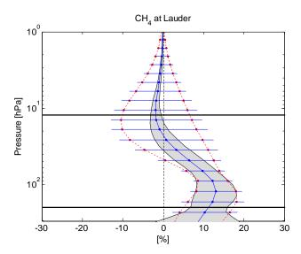
**Fig. 15e.** Statistical means and standard deviations of the relative differences mean(MIPAS-FTIR)/mean(FTIR) [%] of the CH<sub>4</sub> profiles measured at Lauder. The shaded areas correspond to the estimated random error on the relative differences. The two black horizontal bars show the pressure ranges used for the partial column comparisons of Table 3.
