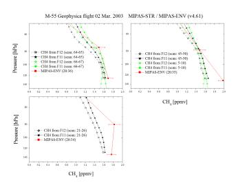
**Fig. 9b.** MIPAS-E CH<sub>4</sub> profiles produced by IPR v4.61 and MIPAS-STR measurements acquired on 03 Mach 2003 from the M-55.
