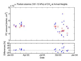
**Fig. 14f.** Time series of CH<sub>4</sub> partial column comparisons. Upper panel: ground-based FTIR (circles) and MIPAS v4.61 (stars) CH<sub>4</sub> partial columns for collocated measurements at Arrival Heights. Lower panel: relative differences between ground-based FTIR and MIPAS partial columns.
