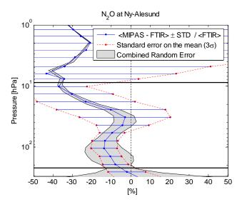
**Fig. 17a.** Statistical means and standard deviations of the relative differences mean(MIPAS-FTIR)/mean(FTIR) [%] of the  $N_2O$  profiles measured at Ny-Alesund. The shaded areas correspond to the estimated random error on the relative differences. The two black horizontal bars show the pressure ranges used for the partial columns of Table 4.
