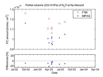
Fig. 16a. Time series of  $N_2O$  partial columns comparisons. Upper panel: ground-based FTIR (circles) and MIPAS v4.61 (stars)  $N_2O$  partial columns for collocated measurements at Ny-Alesund. Lower panel: relative differences between ground-based FTIR and MIPAS partial columns.
