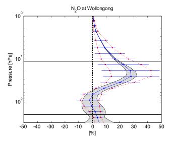
**Fig. 17d.** Statistical means and standard deviations of the relative differences mean(MIPAS-FTIR)/mean(FTIR) [%] of the  $N_2O$  profiles measured at Wollongong. The shaded areas correspond to the estimated random error on the relative differences. The two black horizontal bars show the pressure ranges used for the partial columns of Table 4. The statistics shown is for the  $\pm 4$  h and  $\pm 400$  km coincidence criteria.
