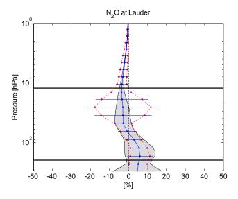
**Fig. 17e.** Statistical means and standard deviations of the relative differences mean(MIPAS-FTIR)/mean(FTIR) [%] of the N<sub>2</sub>O profiles measured at Lauder. The shaded areas correspond to the estimated random error on the relative differences. The two black horizontal bars show the pressure ranges used for the partial columns of Table 4.
