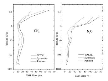
**Fig. 1.** Random, systematic and total errors for the nominal sets of microwindows used in off-line processing in normal MIPAS operations for CH<sub>4</sub> (left panel) and N<sub>2</sub>O (right panel), and for a global composite of results for the five reference atmospheres, with twice the weight given to results from the polar winter case.
