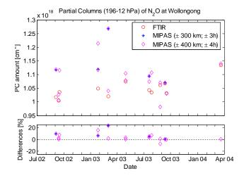
**Fig. 16d.** Time series of  $N_2O$  partial columns comparisons. Upper panel: ground-based FTIR (circles) and MIPAS v4.61 (stars)  $N_2O$  partial columns for collocated measurements at Wollongong. Lower panel: relative differences between ground-based FTIR and MIPAS partial columns.
