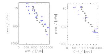
**Fig. 5a.** Comparison of MIPAS CH<sub>4</sub> v4.61 profiles (blue triangles) with the Bonbon cryosampler (gray circles) on 24 September 2002. The left panel is a direct comparison with 3 nearest MIPAS profiles for the same day. The right panel displays 5 days backward and forward trajectory transported profiles matching the cryosampler profile for a larger statistics.
