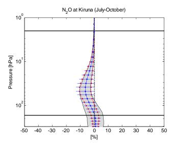
**Fig. 17b.** Statistical means and standard deviations of the relative differences mean(MIPAS-FTIR)/mean(FTIR) [%] of the  $N_2O$  profiles measured at Kiruna. The shaded areas correspond to the estimated random error on the relative differences. The two black horizontal bars show the pressure ranges used for the partial columns of Table 4.
