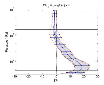
**Fig. 15c.** Statistical means and standard deviations of the relative differences mean(MIPAS-FTIR)/mean(FTIR) [%] of the CH<sub>4</sub> profiles measured at Jungfraujoch. The shaded areas correspond to the estimated random error on the relative differences. The two black horizontal bars show the pressure ranges used for the partial column comparisons of Table 3.
