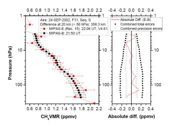
**Fig. 3a.** Comparison of MIPAS CH<sub>4</sub> v4.61 profile with MIPAS-B on 24 September 2002 with MIPAS-B minus MIPAS-E v4.61 differences and combined error bars on the left.
