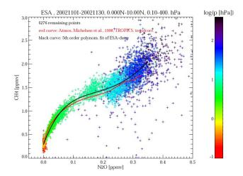
**Fig. 21.** ESA MIPAS  $CH_4$  and  $N_2O$  data plotted against each other and compared with  $CH_4$ - $N_2O$ -regression-curves fitted to ATMOS  $(2002/11/01-2002/11/30, 0.000^{\circ}N-10.00+N)$ .
