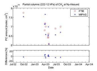
**Fig. 14a.** Time series of  $CH_4$  partial column comparisons. Upper panel: ground-based FTIR (circles) and MIPAS v4.61 (stars)  $CH_4$  partial columns for collocated measurements at Ny-Alesund. Lower panel: relative differences between ground-based FTIR and MIPAS partial columns.
