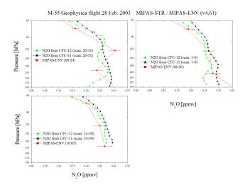
**Fig. 10a.** MIPAS-E  $N_2O$  profiles produced by IPR v4.61 and MIPAS-STR measurements acquired on 28 February 2003 from the M-55.
