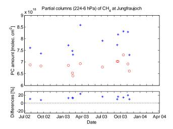
**Fig. 14c.** Time series of CH<sub>4</sub> partial column comparisons. Upper panel: ground-based FTIR (circles) and MIPAS v4.61 (stars) CH<sub>4</sub> partial columns for collocated measurements at Jungfraujoch. Lower panel: relative differences between ground-based FTIR and MIPAS partial columns.
