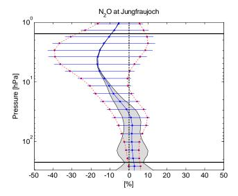
**Fig. 17c.** Statistical means and standard deviations of the relative differences mean(MIPAS-FTIR)/mean(FTIR) [%] of the N<sub>2</sub>O profiles measured at Jungfrau. The shaded areas correspond to the estimated random error on the relative differences. The two black horizontal bars show the pressure ranges used for the partial columns of Table 4.
