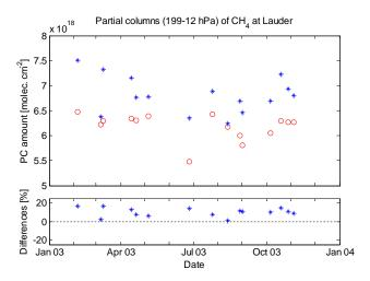
**Fig. 14e.** Time series of CH<sub>4</sub> partial column comparisons. Upper panel: ground-based FTIR (circles) and MIPAS v4.61 (stars) CH<sub>4</sub> partial columns for collocated measurements at Lauder. Lower panel: relative differences between ground-based FTIR and MIPAS partial columns.
