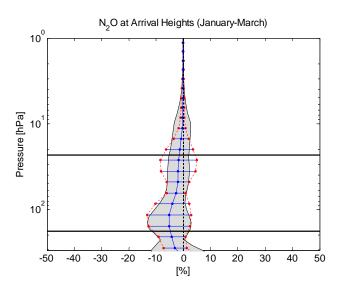
**Fig. 17f.** Statistical means and standard deviations of the relative differences mean(MIPAS-FTIR)/mean(FTIR) [%] of the N<sub>2</sub>O profiles measured at Arrival Heights. The shaded areas correspond to the estimated random error on the relative differences. The two black horizontal bars show the pressure ranges used for the partial columns of Table 4.
