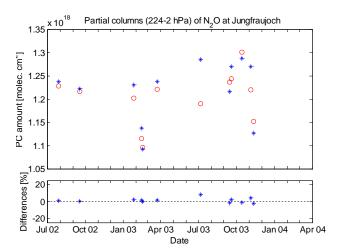
**Fig. 16c.** Time series of  $N_2O$  partial columns comparisons. Upper panel: ground-based FTIR (circles) and MIPAS v4.61 (stars)  $N_2O$  partial columns for collocated measurements at Junhgfraujoch. Lower panel: relative differences between ground-based FTIR and MIPAS partial columns.
