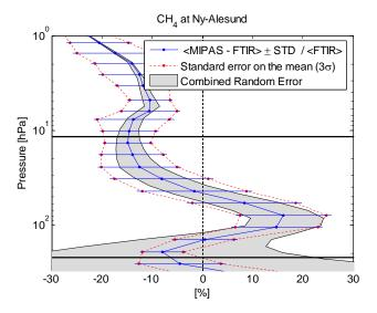
**Fig. 15a.** Statistical means and standard deviations of the relative differences mean(MIPAS-FTIR)/mean(FTIR) [%] of the  $CH_4$  profiles measured at NY-Alesund. The shaded areas correspond to the estimated random error on the relative differences. The two black horizontal bars show the pressure ranges used for the partial column comparisons of Table 3.
