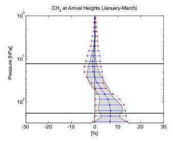
**Fig. 15f.** Statistical means and standard deviations of the relative differences mean(MIPAS-FTIR)/mean(FTIR) [%] of the  $CH_4$  profiles measured at Arrival Heights. The shaded areas correspond to the estimated random error on the relative differences. The two black horizontal bars show the pressure ranges used for the partial column comparisons of Table 3.
