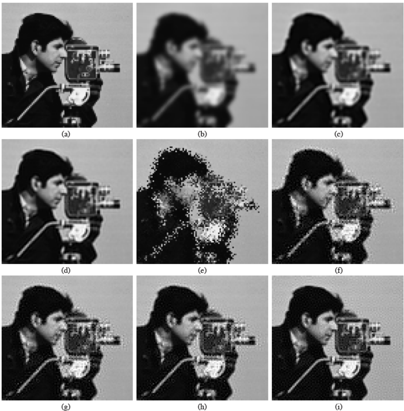
Fig. 7. Images obtained after 9 rotations of angle 2\pi/9 on a part of the camera image depicted in (a), using (b) bilinear, (c) bicubic and (d) O-MOMS interpolation, and our method in three shears with filters (e) h_\tau^0 (nearest neighbor), (f) h_\tau^{1,1} , (g) h_\tau^{1,2} , (h) h_\tau^{1,3} , (i) h_\tau^\infty (sinc). The PSNRs are from (b) to (i): 21.19, 25.15, 29.77, 15.63, 23.07, 25.05, 26.02, 28.67 dB, respectively. The images obtained with h_\tau^{2,2} , h_\tau^{2,3} and h_\tau^{2,4} , not reproduced here, give PSNRs of 26.07, 27.24 and 27.93 dB, respectively.
